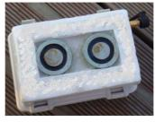
(a) 10 kg capacity one-directional magnet (b) Bottom of the leaf nodes Fig. 12 Magnet-based sensor attachment
