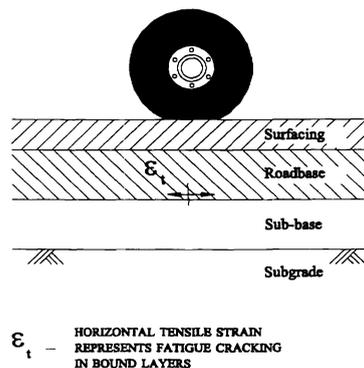
**Figure 1, Section through a thinner asphalt pavement showing mechanism of fatigue cracking**
