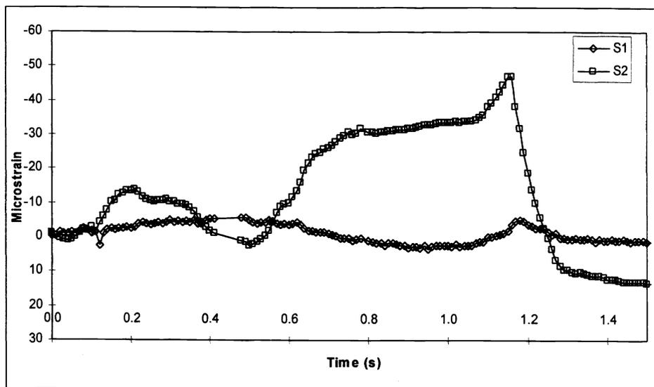
**Figures 10(a) and 10(b):** Graphs of Packet Number and Strain under a loaded truck (40kN wheelload) travelling at 65km/h
