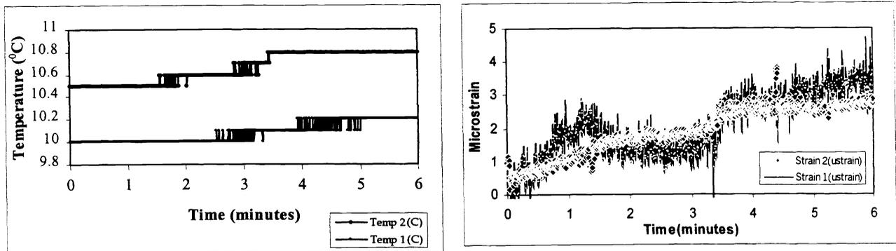
Figure 8(a) and 8(b): Plot of Strain and Temperature In-Situ with no Traffic
