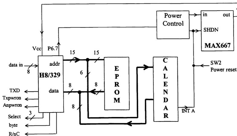
Figure 5: Processor Board
