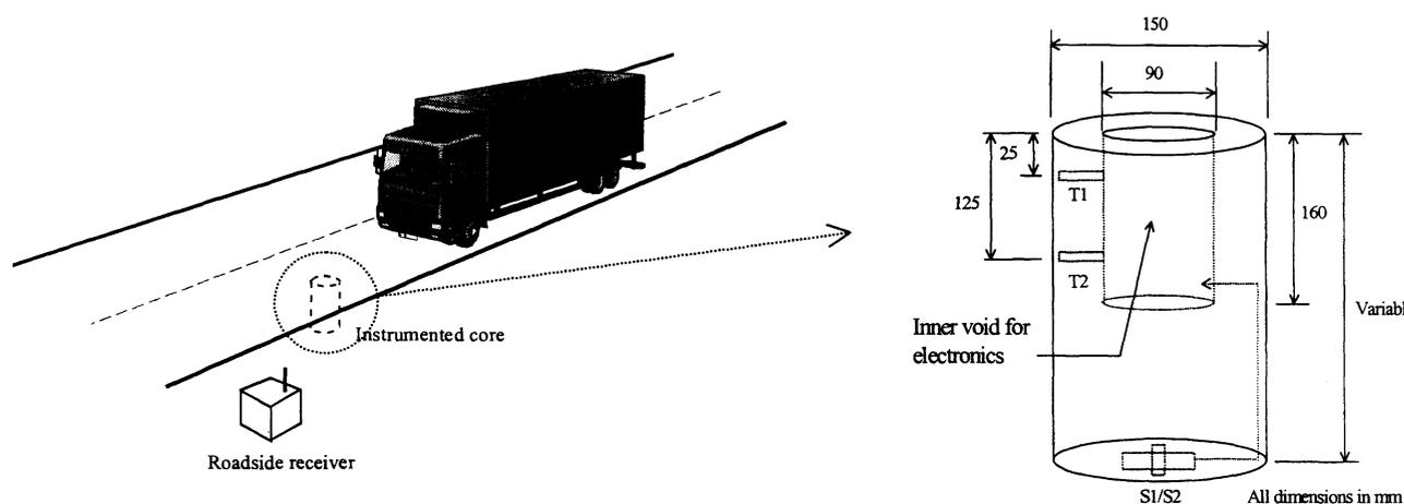
Figure 2, Overview of the instrumented core and wireless system
